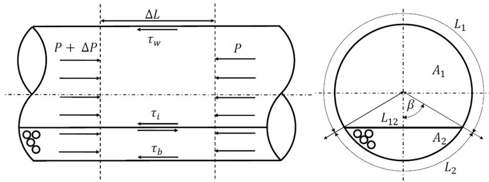
Figure 1. Generic definition sketch for two layer model (Fraser & Goosen, 2018)
