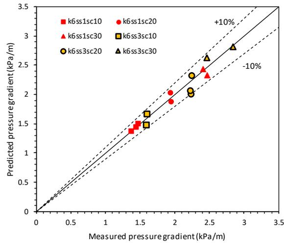
Figure 3. Parity plot comparing measured experimental data points and the two-layer model predicted data.
