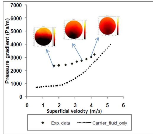
Figure 4. Pressure gradient with concentration profile from ERT (Kabengele et al., 2012)
