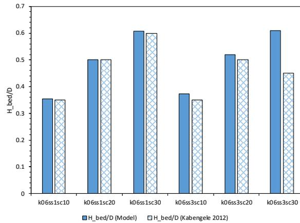
Figure 5. Comparison of the bed depth to pipe diameter ratio from ERT measurements to Two-layer predicted bed depth to pipe diameter ratio.
