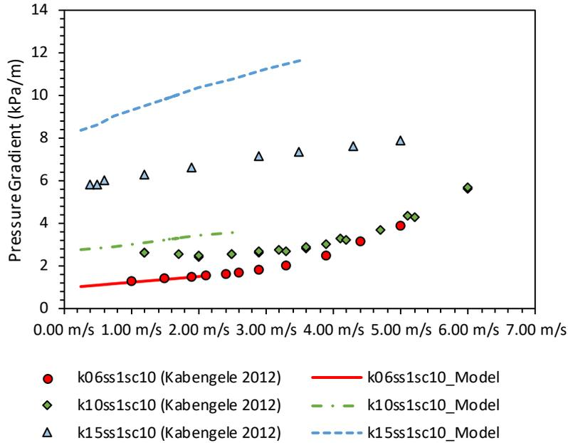
Figure 2. Typical two-layer predictions for the experimental results from Kabengele et al., (2012)
